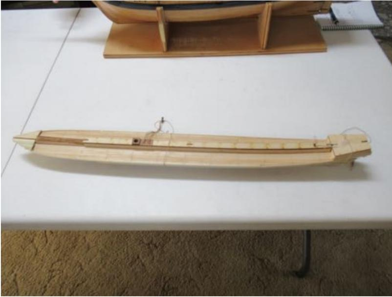
Don was next up to talk about his progress (very slow) on the *Le Real*. Don is still installing the first layer of planking on the model, which is different from all other ship model plank-on-bulkhead kits Don has built in the past. The stem, keel and sternpost are installed AFTER both layers of planking are installed. Don is installing the first layer of strakes with no particular regard to position, as he does not
